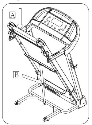
Support place A with hand, kick the place of air pressure bar, then the base frame will fall down automatically (Please keep anybody and any pet away the machine when falling down).
