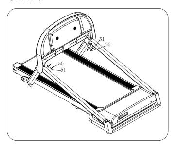
1. Hold on the Computer frame and use the 5# Allen wrench(45), bolt(50) and lock washer (51), fix the computer frame onto the right and left upright.
