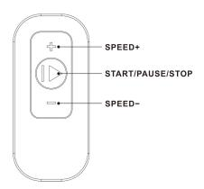
The remote control is a three-button remote control, the upper key is "Speed +", the lower key is "Speed -", the middle key is "Start / Pause / Stop" and press once to start running, then press once again to pause and hold for three seconds to stop running.
