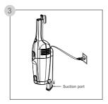
If you need to adjust the length of the dust collection suction port during use, pull it out from the suction port.
