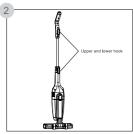
After the product has been used, the power cord can be wrapped around the upper and lower hooks.
