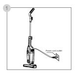
Please make sure that all parts of the machine have been installed before use, and that the power cord is removed from the upper and lower hooks and inserted into the power outlet.
