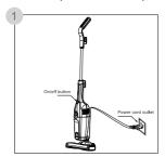
Turn off the power on/off switch of the machine and then unplug it from the power outlet.
