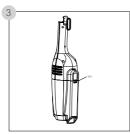
Assemble the dust box to the machine, align the latch at the back and push up, the installation is successful when you hear a click at the latch.
