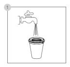
Remove the hepa from the dust box and gently pat it clean, then rinse the hepa with cold water.
