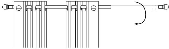
3. Place left bracket in upper left corner of the window recess and extend the pole to right hand corner.
