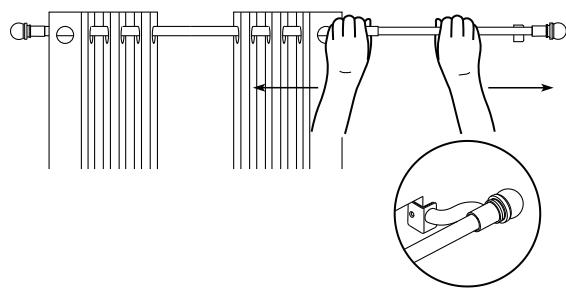
4. With a hand on each pole, push the poles outwards applying firm pressure in both directions to brace against each wall. To finally tension the pole, twist the thin rod away from you (see sticker number 2 on pole).
