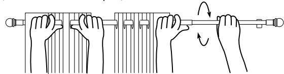
5. Twist right hand end finial away from you until resistance is felt. This tension allows the pole and the brackets to fit flush to the wall. Remove stickers after completing installation.
