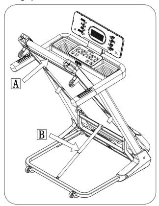
Pull up the main frame at position (A) till hearing the sound that the air pressure bar (B) is locked into the round tube.
