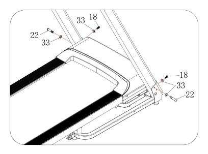
1.Use 5# Allen wrench, firstly lock upright onto base frame by bolt (22) and lock washer (33), then lock upright onto base frame by bolt (18) and lock washer (33).
