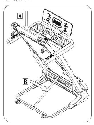
Support place A with hand, kick the place of air pressure bar, then the main frame will fall down automatically. (Please keep anybody and any pet away the machine when falling down).
