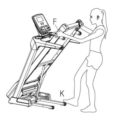
To tilt, start by placing one hand at position "F" to support the top end of the treadmill. Next, place one foot at position "K" to hold the bottom end of the treadmill steady. With your foot at "K", slowly tilt the top of the treadmill downward towards the ground. Once the Main Frame "F" reaches a low enough point, the wheels of the treadmill will become active.
