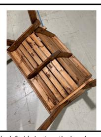
To attach the left side leg turn the bench over, insert 5 bolts in the pre-drilled holes of the left leg and position on the back and base. Secure with nut and washer on each bolt.
