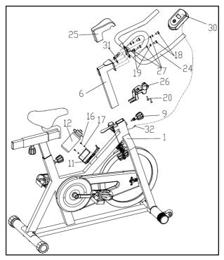
Insert the Meter (30) onto the Meter bracket (31), and then insert the Sensor wire (32) into the hole on the back of Meter (30).
